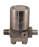
The Ruelco FV-1 is designed to remove the hydraulic signal to a surface controlled subsurface safety valve in the event of a fire and stop any well fluid returns due to packing leaks in the SSCSV. It can also act as a BOP and provides protection from well fluid returns through the control line during normal operating conditions.
